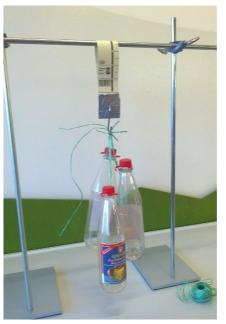
It might happen that the strips of paper will be damaged before the glue joint fails. This tells us that the glue is sufficient for its purpose – gluing paper.
