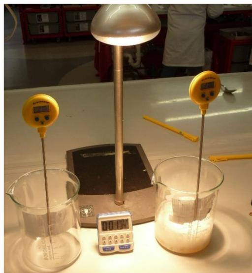
The construction must be symmetrical, i.e. the beakers and thermometers must have the same distance from the lamp.
