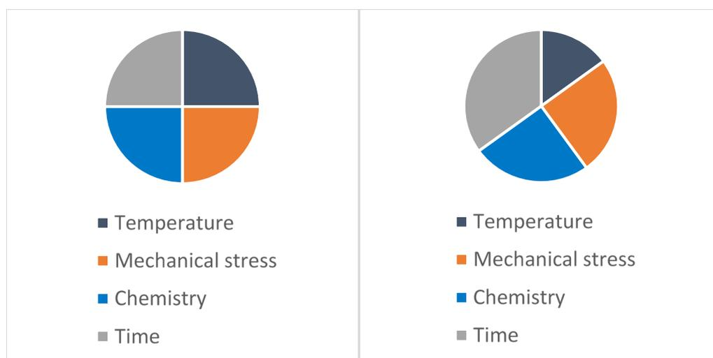
The Sinner’s circle is the underlying principle of the laundry experiments. Additionally, the basic ingredients of detergents plus the effect of the amount of water can also be investigated.
