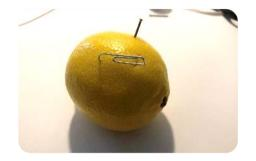
**Insert an iron nail and a copper paper clip into a** lemon. Bend the paper clip so that the wire is straight at one end and remains bent at the other end. Insert the long, straight end into the lemon.
